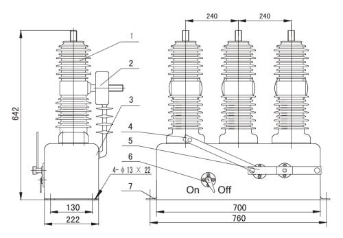
1.Pole 2.CT 3.Frame 4.Handle 5.Manual charging rod 6.On/off indicator 7.Installation plate
